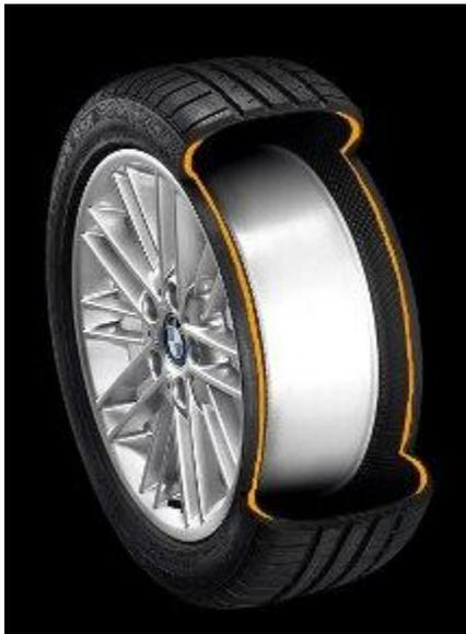
Run flat tyres, as the name suggests, are capable of limited operation when deflated. They are typically only fitted to certain models in certain manufacturer's ranges. Apart from the obvious advantage, their use can allow the vehicle manufacturer to dispense with the spare wheel. Disadvantages are that replacements may not be immediately available, they cost more, they require special tooling to remove and refit and because they have a much stiffer side wall, ride quality can be compromised.
