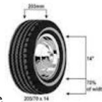
You must never fit wheels and tyres of different size or profile to the same axle except when a 'space-saver' or 'emergency-use' spare tyre supplied by the vehicle manufacturer is in use. These tyres are for emergency use only and information regarding speed and any other restrictions that apply to their use is contained in the owner's handbook, on the spare wheel and on the tyre placard.
